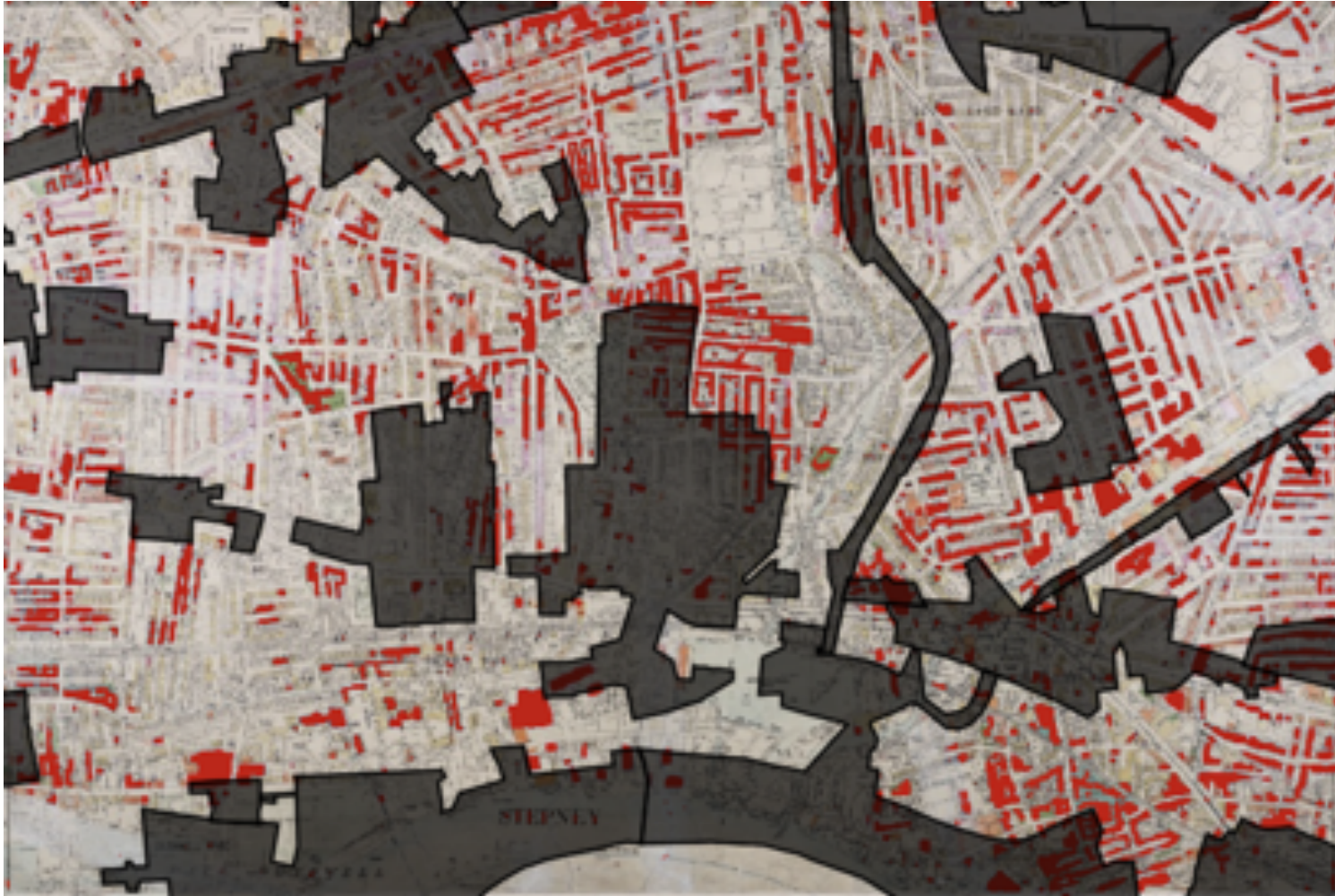
Figure 3: Illustration of bomb damage data extracted from historic hand color coded maps using a random forest classifier
