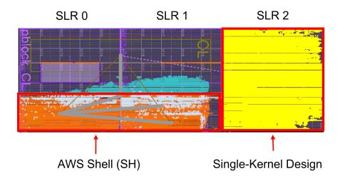
Note: Resources utilized by: (i) the single-kernel CL design (yellow area); (ii) by the AWS Shell (orange area); and (iii) available CL resources (other colors). The image is captured using Xilinx Vivado.
