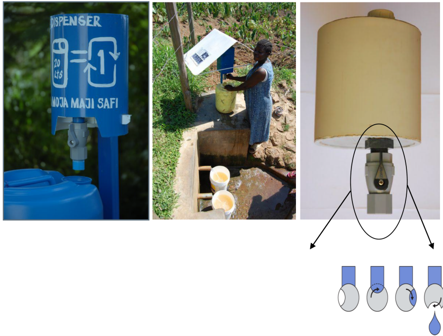
Figure 1: The Chlorine Dispenser
